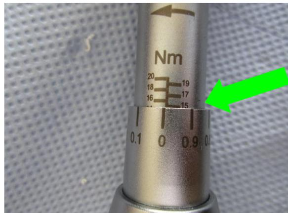
**Prepare the torque wrench by setting at 15 Nm, push the ring with the fingers back, to unlock and turn with the other hand the spindle until the 15Nm shows up.**
