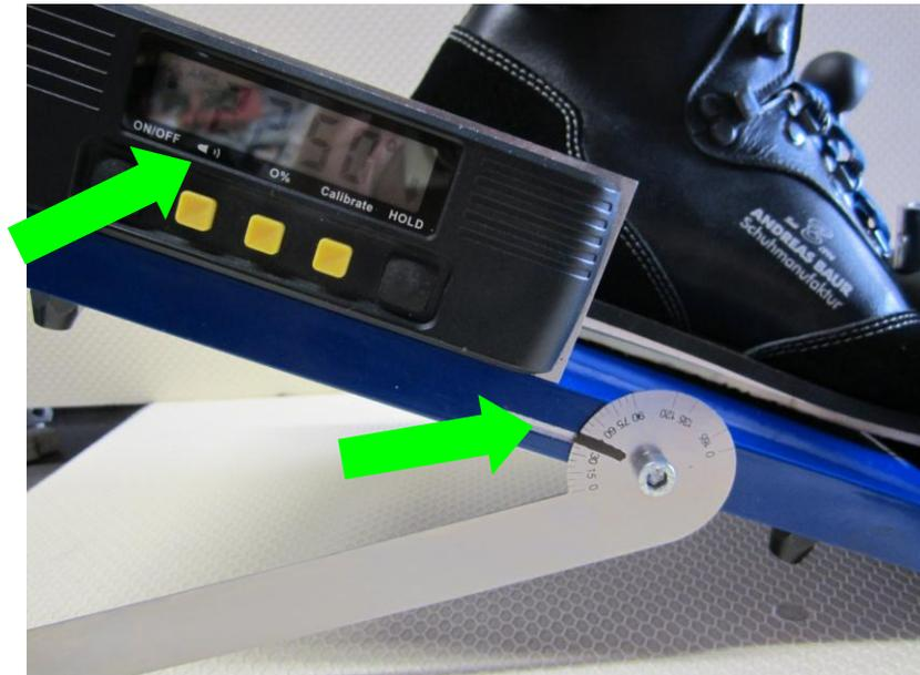
**4. Switch on the digital display. The display will show the angle in degrees. The alternative, but less accurate, measure, is the rule attached to the side of the Tester. There are marks on the rule and on the side of the Tester. When these marks are in line, this means that the boot has achieved an angle of 22.5 degrees.**
