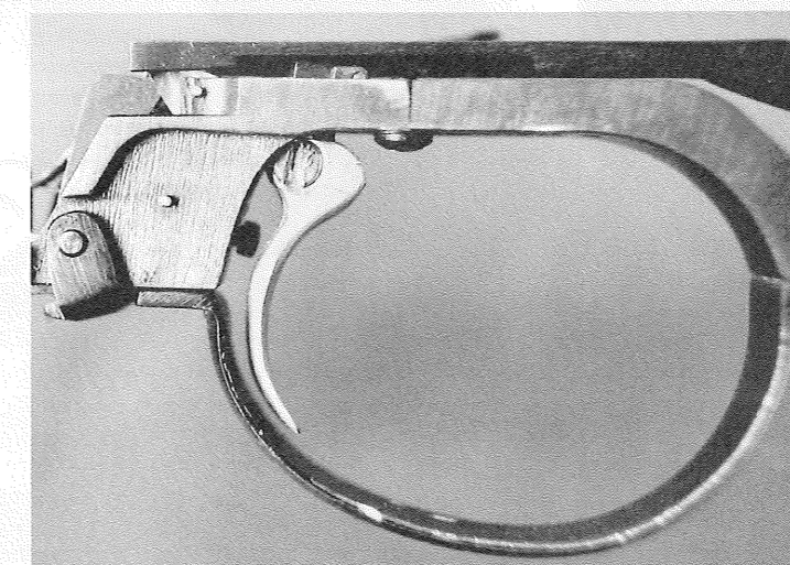
The secret of the Toz is concealed behind the trigger and above it: the jolt-free shot release and rotating trigger.
