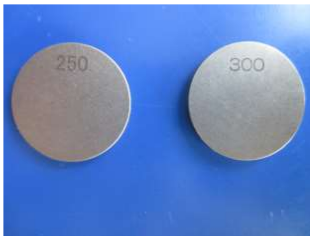
Mess shims for thickness and stiffness device
