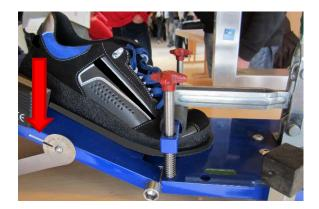
Switch on the digital display. The display will show the angle in degrees. The alternative, but less accurate, measure, is the rule attached to the side of the Tester. There are marks on the rule and on the side of the Tester. When these marks are in line, this means that the boot has achieved an angle of 22.5 degrees. Insert the torque wrench and push it down until it 'clicks'. Boots should have a minimum angle of 22.5 degrees.
