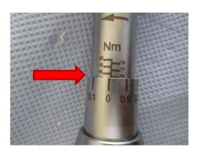
Prepare the torque wrench by setting at 15 Nm, push the ring with the fingers back, to unlock and turn with the other hand the spindle until the 15 Nm shows up.
