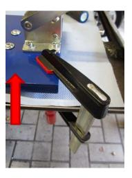
Fix the Tester on to a flat surface (a table is ideal) by the clamp (as shown by the red arrow).
