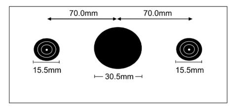
10m Running Target Electronic Target The 30.5mm diameter is a hole.
