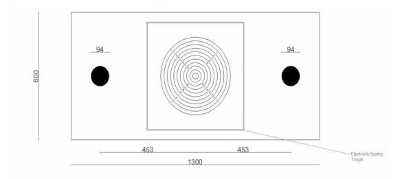
50m Running Target Electronic Target
