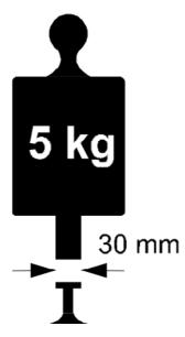
The device used to measure the thickness of clothing and shoes must be capable of measuring to one-tenth of a millimetre (0.1mm). Measurements must be taken with a 5.0kg weight applied. The device must have two (2) circular flat surfaces facing each other, each 30mm in diameter.
